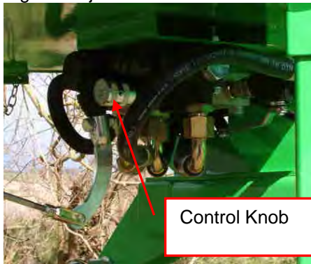
Fig 5.4 Adjustable feed roller control
