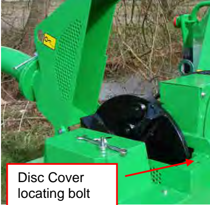
Fig 5.1.2 Chipper Disc Cover
