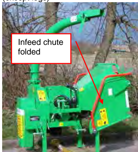
Fig 5.6 Chutes ready for transport (except legs)
